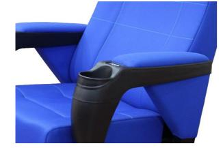
Seatrest and Backrest are manufactured from polyurethane material in aluminum molds which are designed in accordance to the human anatomy and have the standart of 50 ± 10% densty and Mvss 302 fire behaviour. Seatrest and Backrest have a durable inner skeleton made of metal profile. Seatrests are manufactured as to be fixed.
