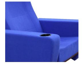
Seatrest and Backrest are manufactured from polyurethane material in aluminum molds which are designed in accordance to the human anatomy and have the standart of  $50 \pm 10$  % densty and Mvss 302 fire behaviour. Seatrest and Backrest have a durable inner skeleton made of metal profile. Seatrests are manufactured as to be fixed.
