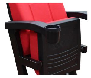
Seatrest and Backrest are manufactured from polyurethane material in aluminum molds which are designed in accordance to the human anatomy and have the standart of  $50 \pm 10\%$  densty and Mvss 302 fire behaviour. Seatrest and Backrest have a durable inner skeleton made of metal profile. Seatrests are manufactured as to have self-closing weight-centered mechanism.
