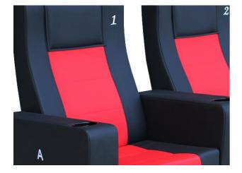
Seatrest and Backrest are manufactured from polyurethane material in aluminum molds which are designed in accordance to the human anatomy and have the standart of  $50 \pm 10$  % densty and Mvss 302 fire behaviour. Seatrest and Backrest have a durable inner skeleton made of metal profile. Seatrests are manufactured as to be fixed.
