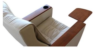
Seatrest and Backrest are manufactured from polyurethane material in aluminum molds which are designed in accordance to the human anatomy and have the standart of  $50 \pm 10$  % densty and Mvss 302 fire behaviour. Seatrest and Backrest have a durable inner skeleton made of metal profile. Seatrests are manufactured as to be fixed.
