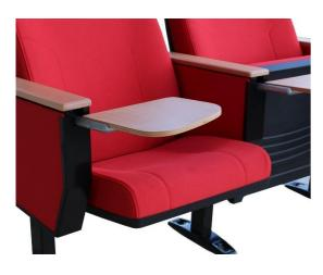
Seatrest and Backrest are manufactured from polyurethane material in aluminum molds which are designed in accordance to the human anatomy and have the standart of 50 ± 10% densty and Mvss 302 fire behaviour.
