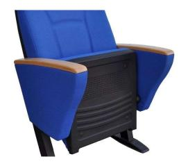
Seatrest and Backrest are manufactured from polyurethane material in aluminum molds which are designed in accordance to the human anatomy and have the standart of  $50 \pm 10\%$  densty and Mvss 302 fire behaviour. Seatrest and Backrest have a durable inner skeleton made of metal profile. Seatrests are manufactured as to have self-closing weight-centered mechanism.
