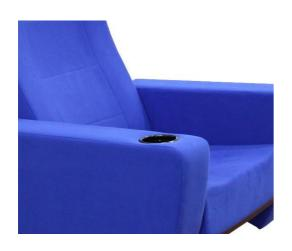
Seatrest and Backrest are manufactured from polyurethane material in aluminum molds which are designed in accordance to the human anatomy and have the standart of 50 ± 10 % densty and Mvss 302 fire behaviour. Seatrest and Backrest have a durable inner skeleton made of metal profile. Seatrests are manufactured as to be fixed.
