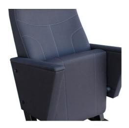
Seatrest and Backrest are manufactured from polyurethane material in aluminum molds which are designed in accordance to the human anatomy and have the standart of 50 ± 10% densty and Mvss 302 fire behaviour. Seatrest and Backrest have a durable inner skeleton made of metal profile. Seatrests are manufactured as to have self-closing weight-centered mechanism.
