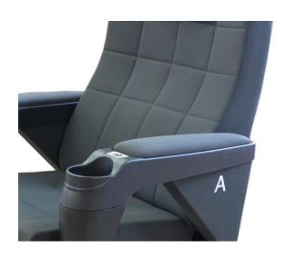
Seatrest and Backrest are manufactured from polyurethane material in aluminum molds which are designed in accordance to the human anatomy and have the standart of 50 ± 10% densty and Mvss 302 fire behaviour. Seatrest and Backrest have a durable inner skeleton made of metal profile. Seatrests are manufactured as to be fixed.
