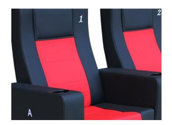
Seatrest and Backrest are manufactured from polyurethane material in aluminum molds which are designed in accordance to the human anatomy and have the standart of 50 ± 10 % densty and Mvss 302 fire behaviour. Seatrest and Backrest have a durable inner skeleton made of metal profile. Seatrests are manufactured as to be fixed.
